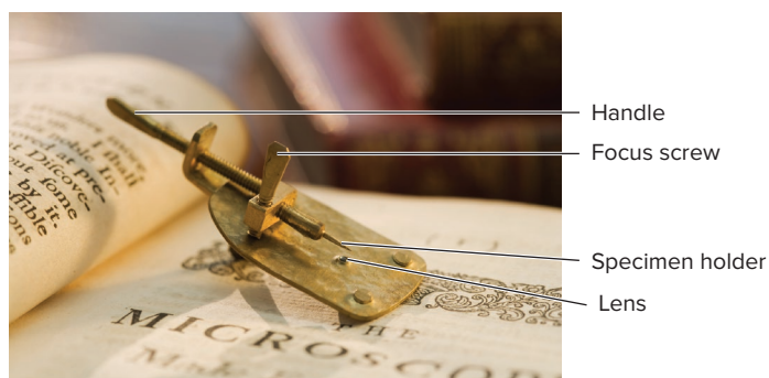
FIGURE 1.1 Model of van Leeuwenhoek's Microscope
